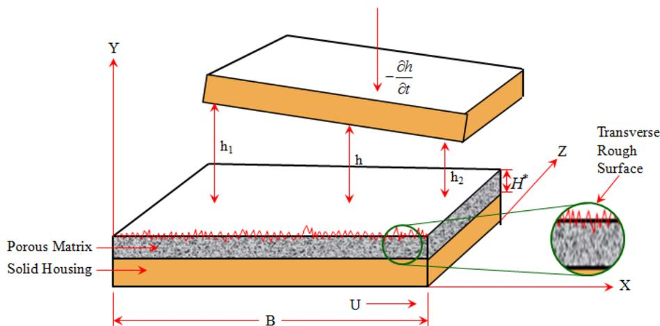
Fig. 1. Physical geometry of porous plane inclined slider bearing
